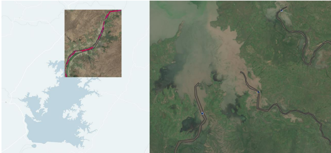
Figure 1: Turbidity retrieval for the Chira river just upstream of the Pochos reservoir (left) and the three tributaries of the Lagdo reservoir (right). For Pochos, the turbidity product is shown, while for Lagdo the true color image is shown
