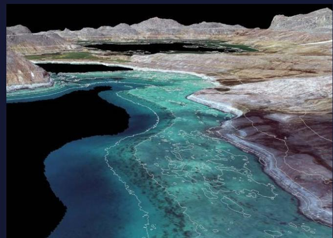
**Digital Twin Horn Island** | A high-resolution digital twin was created using satellite-derived bathymetry, topography, and land classification data to support decision-making in a remote coastal terrain.
